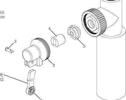
ATTENTION: DO NOT PUT PRESSURE ON VALVE ARM WHILE TIGHTENING FRONT VALVE ASSEMBLY.
